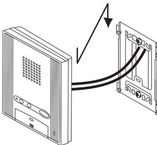
**3** Mount the station unit to the mounting bracket.
