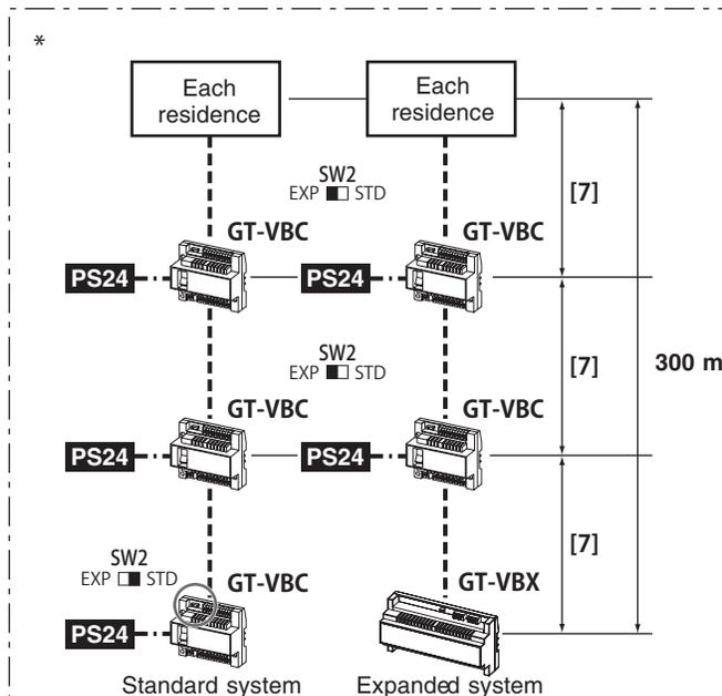
The GT-VBC can be used as an extension adaptor as well (2 units per trunk line). To do so, set the setting switch (SW2) to "EXP". Use the unit as an extension adaptor in expanded systems. Even if two units are used as extension adaptors (SW2: EXP), the wiring distance to the farthest residential station from the GT-VBC (SW2: STD) or GT-VBX is limited to 300 m.
