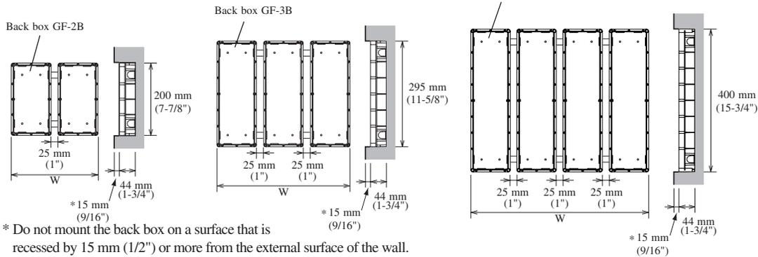
\* Do not mount the back box on a surface that is recessed by 15 mm (1/2") or more from the external surface of the wall.
