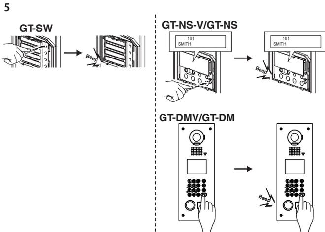
After step 5, press and hold the ⊕ button until the confirmation tone sounds. A beep will sound and the link to the corresponding residential station will be erased.
