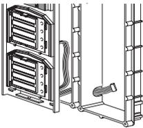
**9** Run the connection cable through the joint pipe (which you should have made open in advance) and connect CN1 of the GT-SW to the next row.
