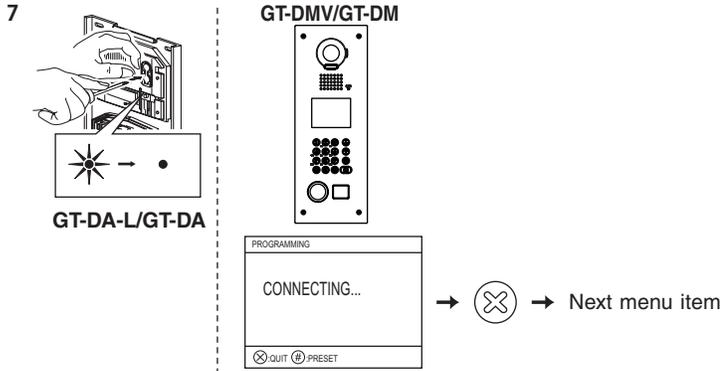
7 Press the program switch of the GT-DA-L/GT-DA to finish programming. The in use LED will go out. For the GT-DMV/GT-DM, press the ⊗ button.
