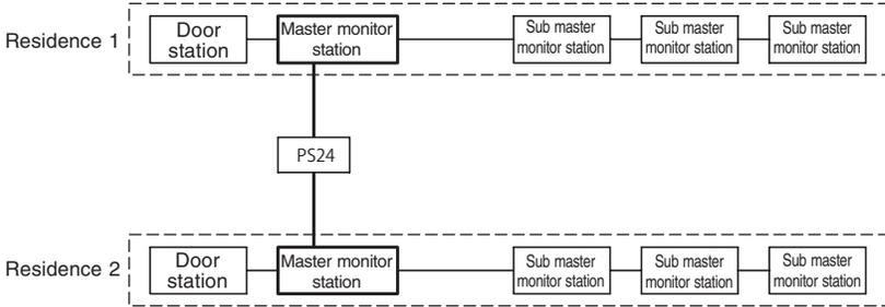
[When sub master monitor stations are not connected]
