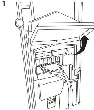
1 Open the cover and connect the wiring to the terminal block.
