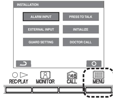
3 To finish changing settings, press the [OFF] button to return to the standby mode. In other cases, set by pressing the [MENU] button. Press the [REC/PLAY] button to cancel the settings and return to the previous screen.
