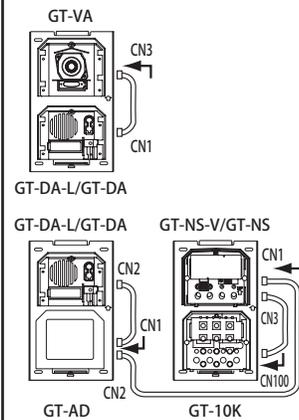
Use the GF-C to connect to the name scrolling module. To position the speech module in the center row, run the GF-C through the joint pipe in advance.
