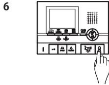
6 Press the OFF button to finish programming. With the handset type module, return the handset. Repeat steps 3 to 6 to program all residential stations.
