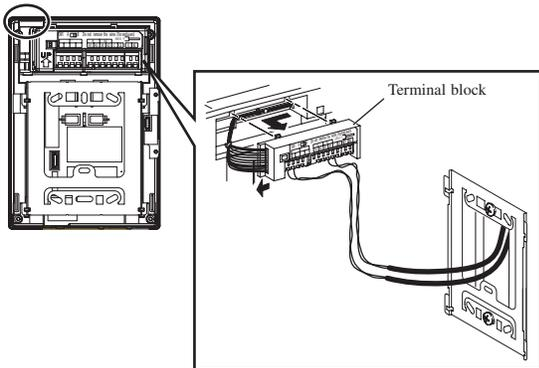
**2** Connect the wiring to the terminal block.
