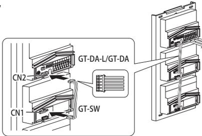
**7** From the speech module to the next module, insert the attached connector into the socket.
