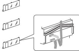
Make sure to run the cable under the terminal cover for protection.
