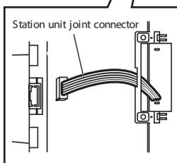
Connect the station unit joint connector.
