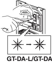
Press the program switch of the GT-DA-L/GT-DA for at least 5 seconds. The in use LED will light up after blinking.
