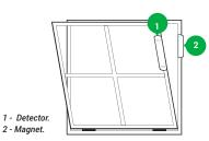
Tilt detector detects the vertical deviation of the device relative to the initial position of more than 5°. DoorProtect Plus can be installed on windows including dormer windows, and the system can be armed, when they are in the airing mode (you should previously disable the magnetic sensor in the settings).
