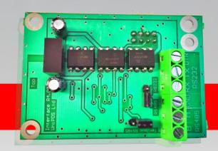
The Interface Module RS232/485 is fully compatible with the FS5100 and FS5200 UniPOS conventional panels. Applicable for PC application and Conventional Network Repeater integration.
