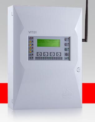
In case of fire event, the results of the combustion are detected from the wireless point fire detector and through radio frequency channel a fire status message is sent to the VIT01 fire control panel. The system components installed at the site are organized into a radio network. The maximum number of independent wireless systems at one premise is 16.
